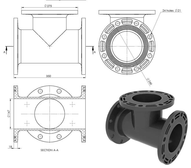
Basic element. Usually, the start point of the connection unit assembly. Flanges 6" let the element connect to the existing pipeline or to another *FORWARD FIT* fitting. Any type of wafer shut-off valves 6" is allowed.
