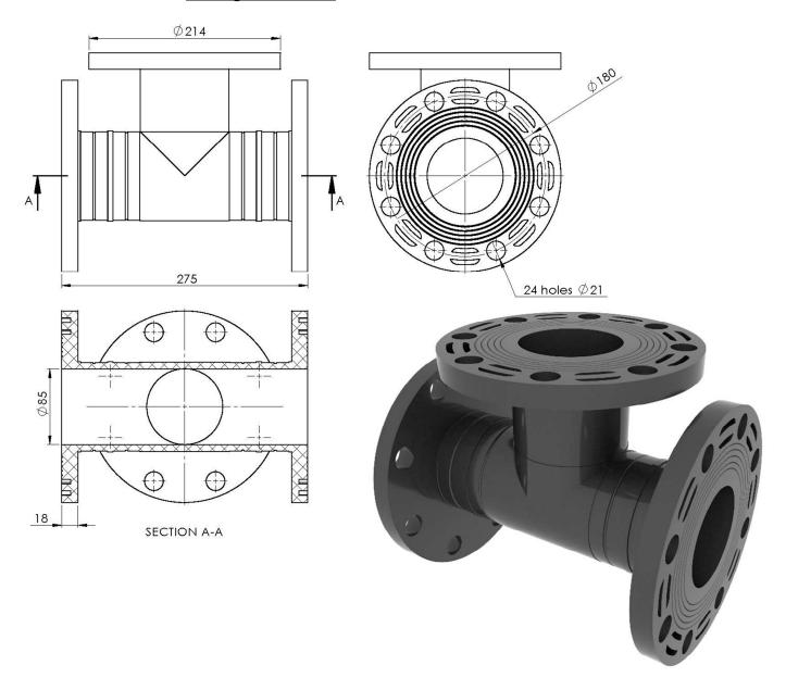
Basic element of the connection unit. Flanges 4" let the element connect to the existing pipeline or to another *FORWARD FIT* fitting. Any type of wafer shut-off valves 4" is allowed.
