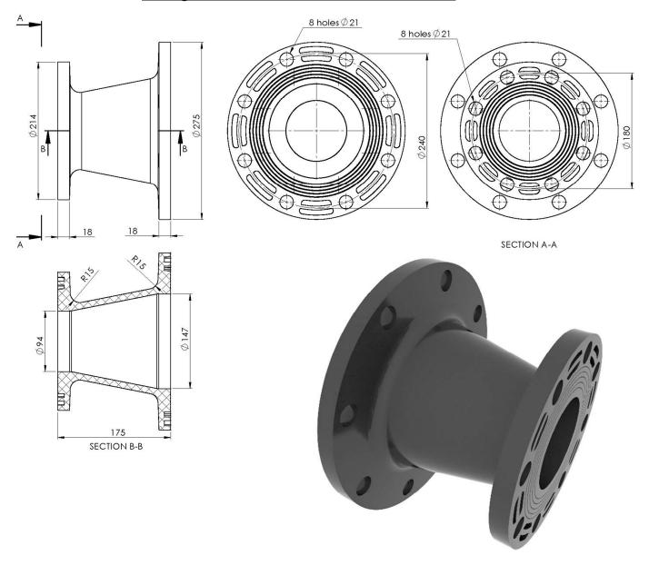
Basic element of the connection unit. Allows the pipeline transition between 6" and 4" diameters. Flanges 6" and 4" let the element connect to the existing pipeline or to another *FORWARD FIT* fitting. Any type of wafer shut-off valves 6" and 4" is allowed.
