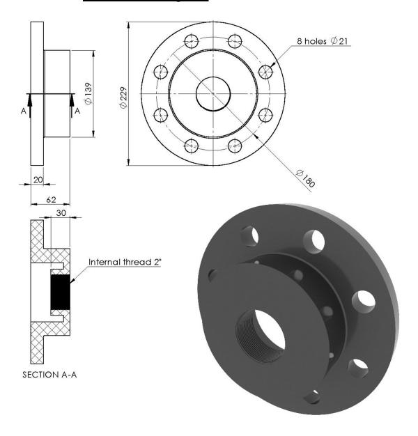
Basic element of the connection unit. Provides any thread 2" elements connection. The thread part diameter can be changed to required one at the customer's request. Flanges 4" let the element connect to the existing pipeline or to another *FORWARD FIT* fitting. Any type of wafer shut-off valves 4" is allowed.
