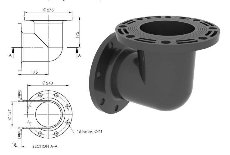
Basic element of the connection unit. Flanges 6" let the element connect to the existing pipeline or to another *FORWARD FIT* fitting. Any type of wafer shut-off valves 6" is allowed.
