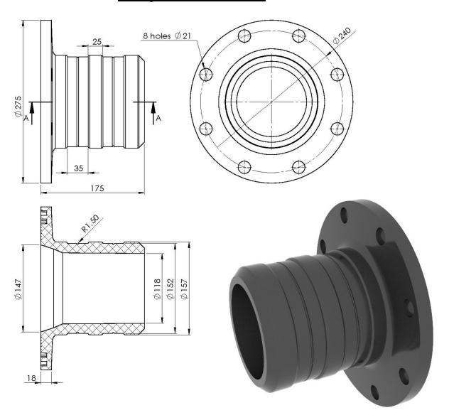
Basic element of the connection unit. Provides flexible pipeline connection. The barb part of the element contains O-rings grooves. Flanges 6" let the element connect to the existing pipeline or to another *FORWARD FIT* fitting. Any type of wafer shut-off valves 6" is allowed.
