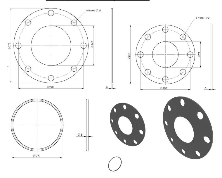
Rubber gaskets for flanges 6" and 4" are used for the inter-flange sealing of *FORWARD FIT* elements' connections.
