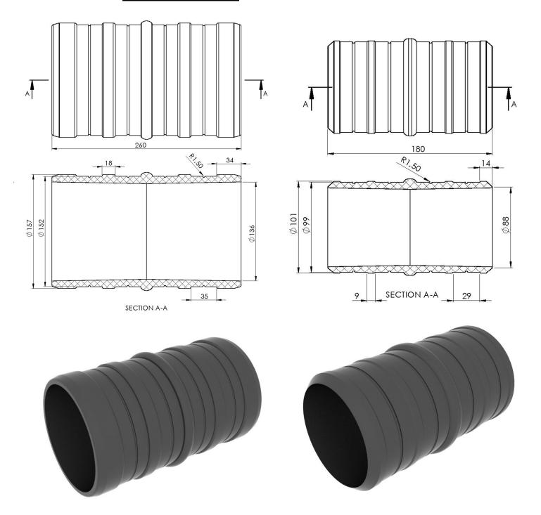
Flexible pipelines' connection element. The barb parts of the elements contain O-rings grooves. The barb part diameter can be changed to required one at the customer's request.
