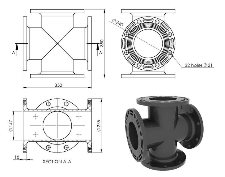
Basic element. Usually, the start point of the connection unit assembly. Flanges 6" let the element connect to the existing pipeline or to another *FORWARD FIT* fitting. Any type of wafer shut-off valves 6" is allowed.
