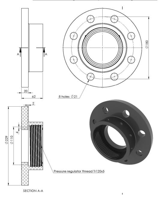
Basic element of the connection unit. Provides pressure regulator 4" connection. Flanges 4" let the element connect to the existing pipeline or to another *FORWARD FIT* fitting. Any type of wafer shut-off valves 4" is allowed.
