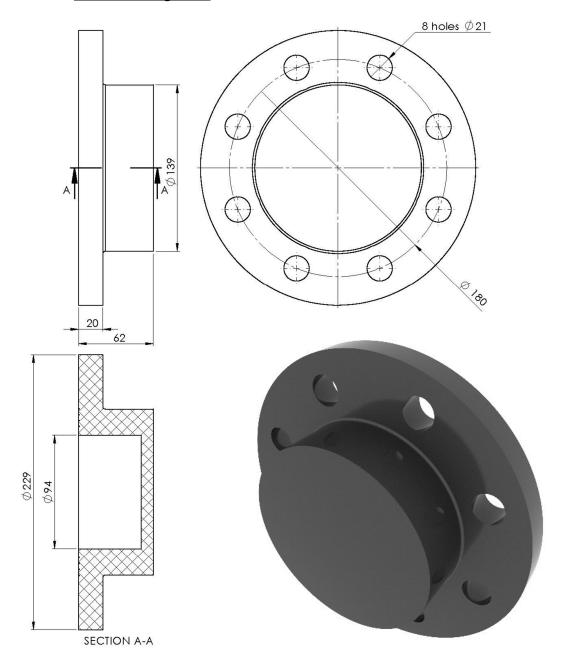
Basic element of the connection unit. Provides the temporarily plugging of the pipeline. Flanges 4" let the element connect to the existing pipeline or to another *FORWARD FIT* fitting. Any type of wafer shut-off valves 4" is allowed.
