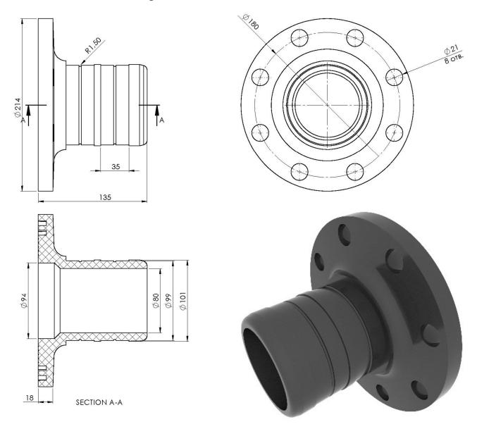
Basic element of the connection unit. Provides flexible pipeline connection. The barb part of the element contains O-rings grooves. The barb part diameter can be changed to required one at the customer's request. Flanges 4" let the element connect to the existing pipeline or to another *FORWARD FIT* fitting. Any type of wafer shut-off valves 4" is allowed.
